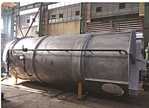
Cooling Bell Mobarake Steel Company
