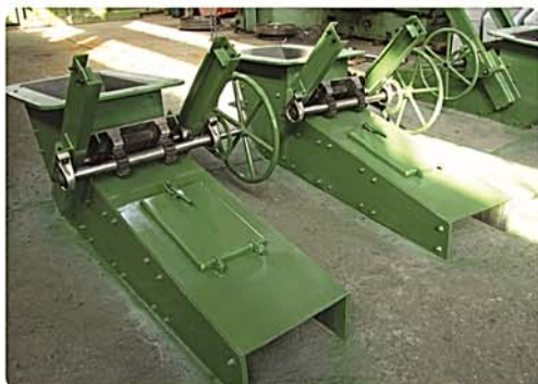
Discharge gate Mobarake Steel Company
