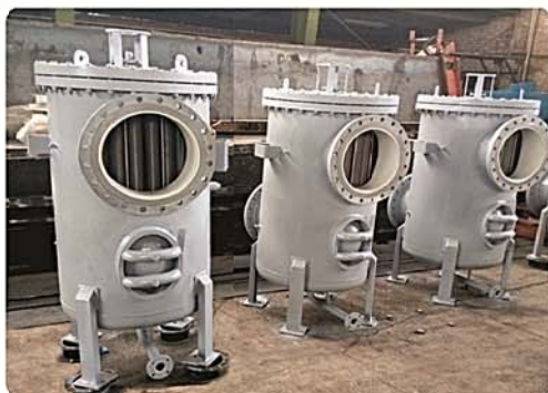
Self Cleaning Filter Mobarake Steel Company
